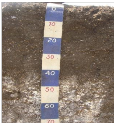
Fig 1: Calcium carbonate accumulated in sub-surface horizon and formation of calcic horizon in arid region of Maharashtra
